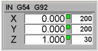
Alternately LZ may be set by shifting MZ the desired amount using G92.1. Using G92.1 it is not necessary to move to the workpiece first.
