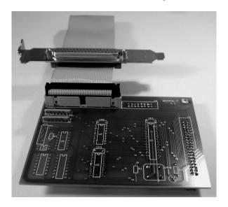
Below is the PCI-7200 card on the left, the Daughter Board on the right and the spacer/screw assembly. Note the matching holes in the Daughter Board and the PCI-7200 card. The small washer is included for a precise fit and must be installed between the boards, at one end of the spacer or the other.
