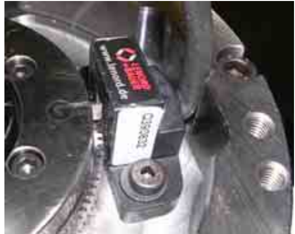
Lenord Bauer magnetic reader (sinusoidal wave)
