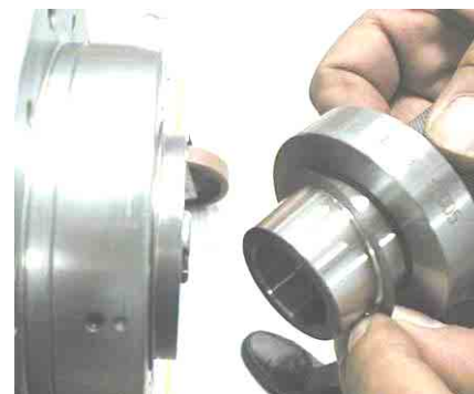
Figure 8.19 interposition of the thickness spacer between the stop surfaces of the gauge and of the spindle shaft
