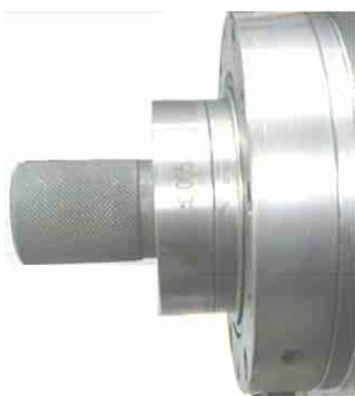
Figure 8.18 use of the gauge as a normal tool-holder, with or without interposed thickness spacer (Figure 8.19), according to the indications of the table shown in the procedures of paragraphs 0 and 0
